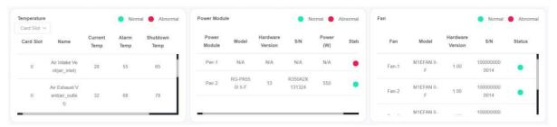
In the **Temperature** panel, you can view the temperature of a card slot by selecting a card clot from the **Card Slot** drop-down list box.
