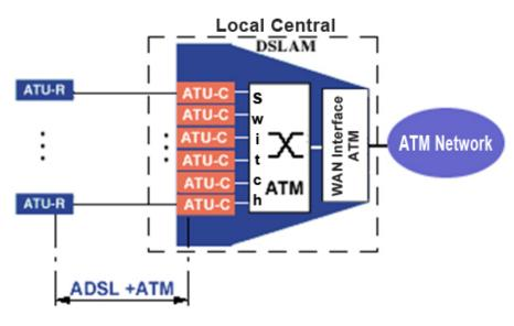
By keeping in mind these advantages, the solution taken to offer services is the transport of ATM cells over an ADSL link (between the ATU-R and ATU-C in DSLAM).
