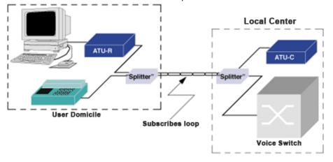
Since this is a modulation where different throughputs are transmitted in User -> Network and Network -> User directions, the ADSL modem at the user end (ATU-R or ADSL Terminal Unit-Remote) is different to the one at the other end of the loop (local central, ATU-C or ADSL Terminal Unit-Central).
